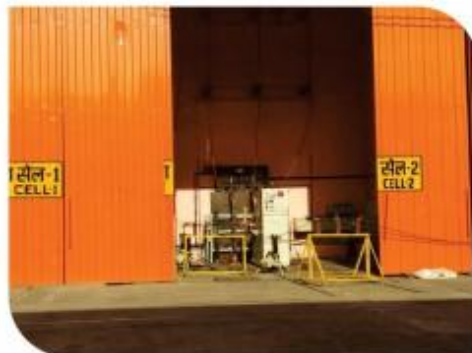
Capacitor bank current switching test of test duties BC1 and BC2 as per IEC: 62271-100, 2012
